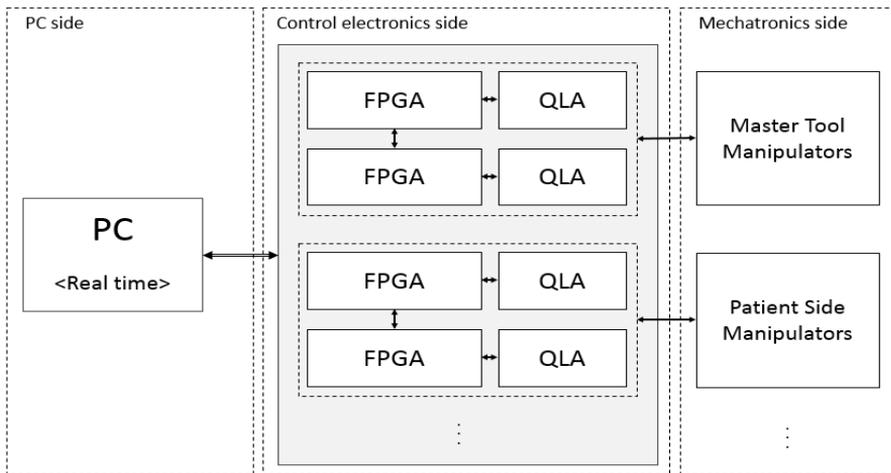
*Figure 3:* Schematic representation of the hardware structure Workstation [32].
