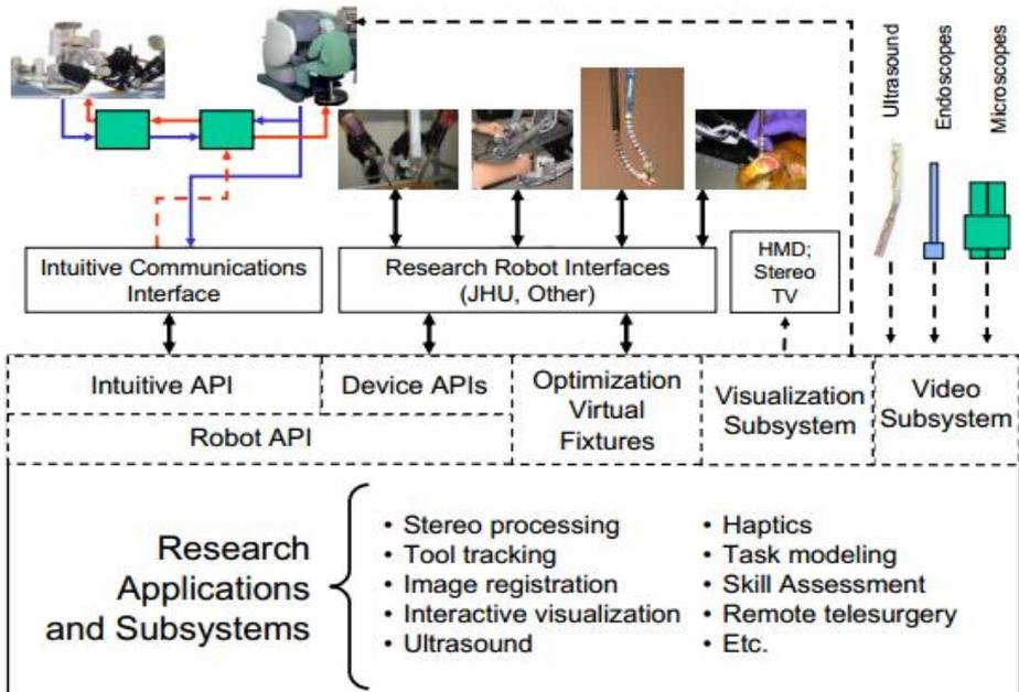
Figure 2: Architecture and capabilities of the Surgical Assistant Workstation [22].
