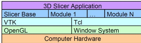
*Figure 1:* The modularity of the 3D Slicer [4].
